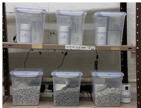
Figure 1. Experimental set up for radon exhalation rate measurements
